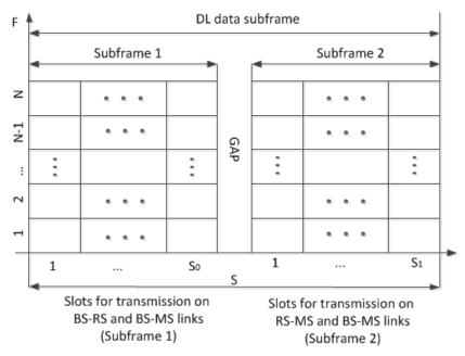
Figure 2. Dowlink data subframe for OFDMA relay-enhanced networks
