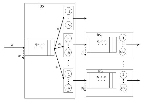
Figure 3. The structure of the model with overall S Chs, which are distributed between BS ans RSs, and K + 1 types of incoming requests
