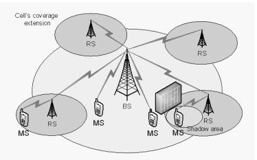
Figure 1. The fixed infrastructure of relay-enhanced LTE-Advanced cellular networks
