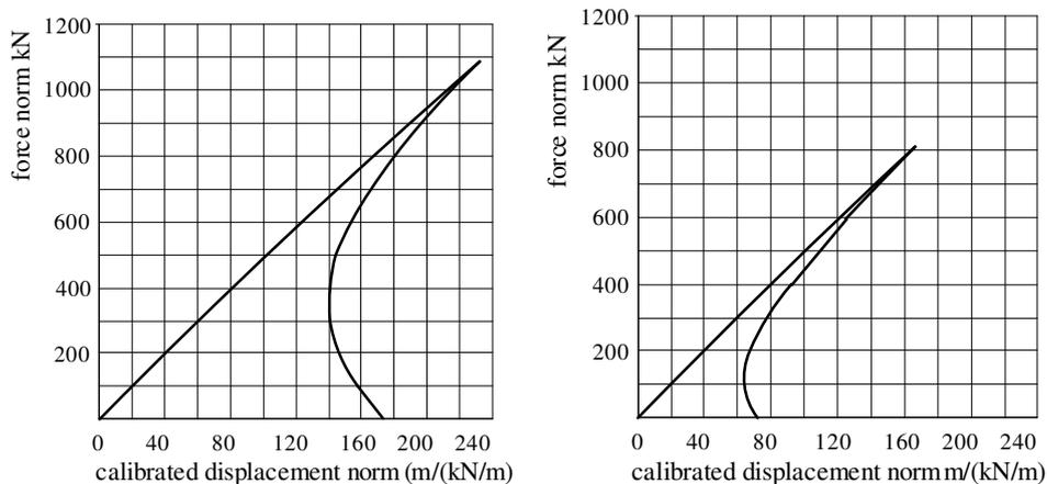
Figure 3. Load paths of the dome in figure 2: (a) Load combination C1; (b) Load combination C2
