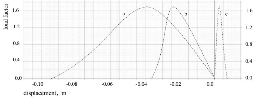
Figure 4. Variation of load factor with displacement at node 42 in the buckling zone for C2 (a) vertical displacement component (b) (c) horizontal displacement components
