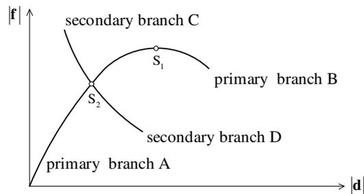
Figure 1. Load path of a structure
