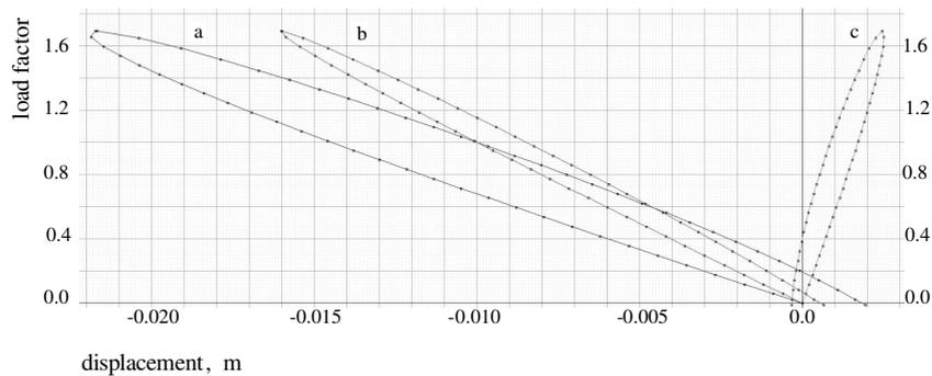
Figure 5. Variation of load factor with displacement at node 74 in the buckling zone for C2 (a) vertical displacement component (b) (c) horizontal displacement components
