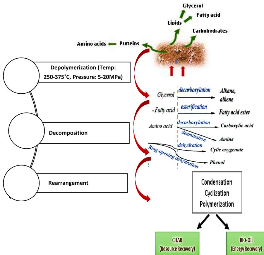
Fig. 3. Reaction pathway of hydrothermal liquefaction of sludge conversion [3,4]
