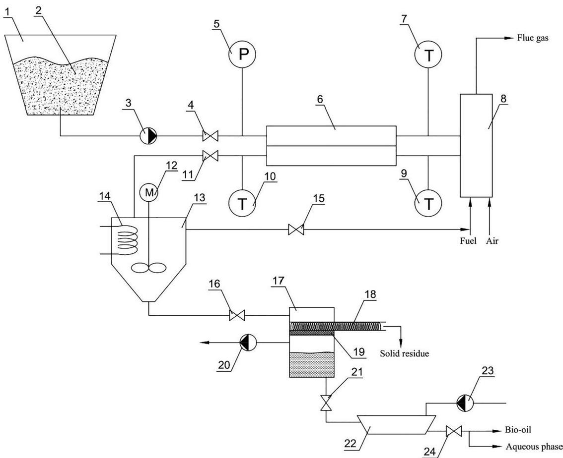
Fig. 4. Schematic representation of hydrothermal liquefaction for thermochemical conversion of sludge to bio-fuel. 1 – bunker, 2 – biomass raw, 3 – high-pressure pump, 4, 11, 15, 16, 21, 24 – valves, 5 – pressure sensor, 6 – heat-exchanger, 7, 9, 10 – temperature sensors, 8 – heater to set temperature, 12 – mixer, 13 – receiver for HTL products, 14 – cooler, 17 – nutsche filter, 18 – screw, 19 – filter, 20 – vacuum compressor, 22 – decanter, 23 – compressor.
