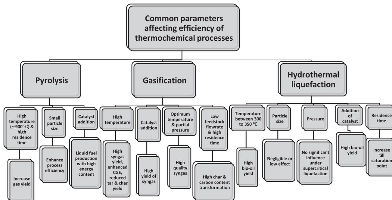
Fig. 9. Common parameters affecting efficiency of thermochemical processes.
