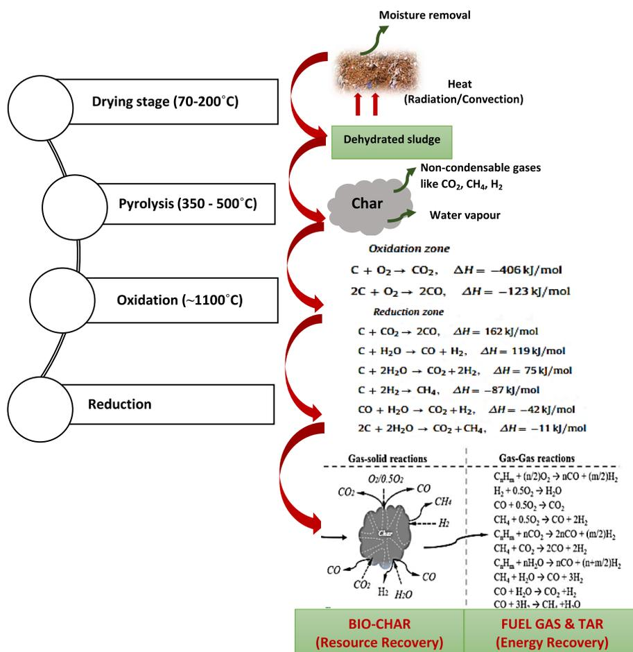
Fig. 7. Reaction pathway of gasification of sludge conversion [3,4]
