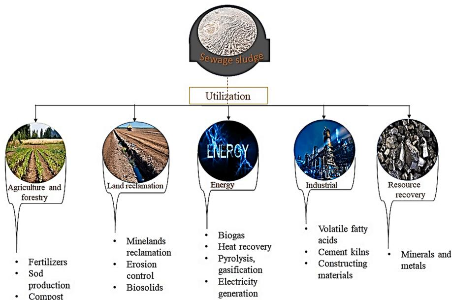
Fig. 1. Utilization of sludge in various sectors.
