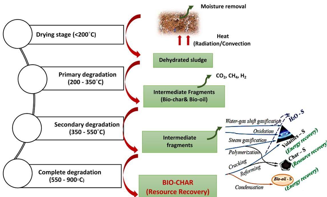
Fig. 5. Reaction pathway of pyrolysis of sludge conversion [3,4]
