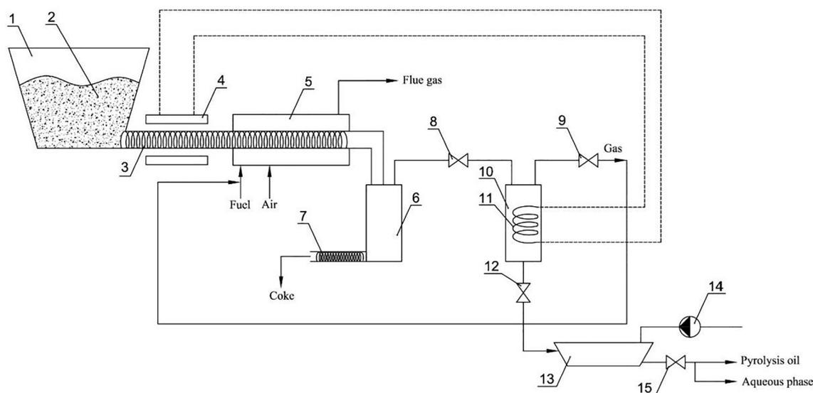
**Fig. 6.** Schematic representation of pyrolysis for thermochemical conversion of sludge to bio-fuel. 1 – bunker, 2 – biomass raw, 3 – feeding screw, 4 – heat-exchanger, 5 – pyrolysis reactor, 6 – receiver for pyrolysis products, 7 – screw, 8, 9, 12, 15 – valves, 10 – receiver for evaporated pyrolysis products, 11 – cooler, 13 – decanter, 14 – compressor.
