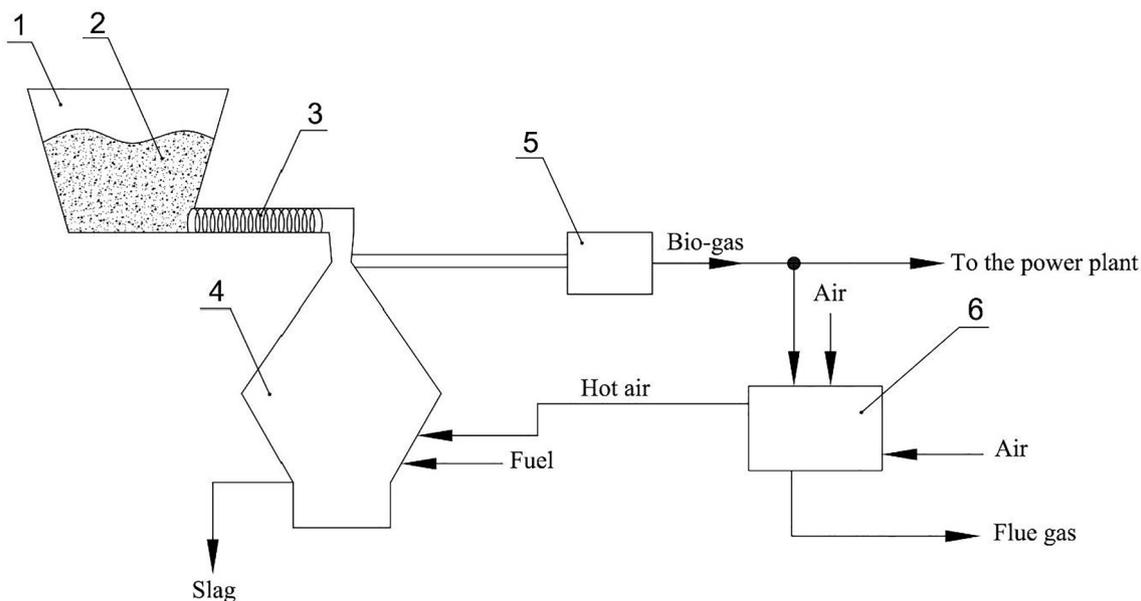
Fig. 8. Schematic representation of gasification for thermochemical conversion of sludge to bio-fuel. 1 - bunker, 2 - biomass raw, 3 - feeding screw, 4 - gasification reactor, 5 - filtering system, 6 - heat-exchanger.
