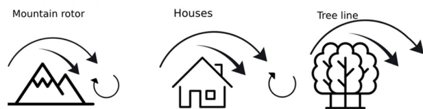
Figure 2. Formation of perturbed air flows near the ground Source: made by A.S. Ermilov, O.A. Saltykova
