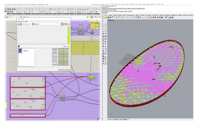
Figure 8. Using the Galapagos solver to optimize sections in the dome
