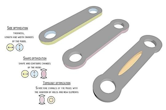
Figure 1. Three types of structural optimization problems
