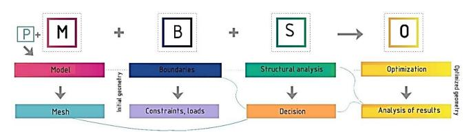
Figure 2. The process of shape optimization in COMSOL Multiphysics
