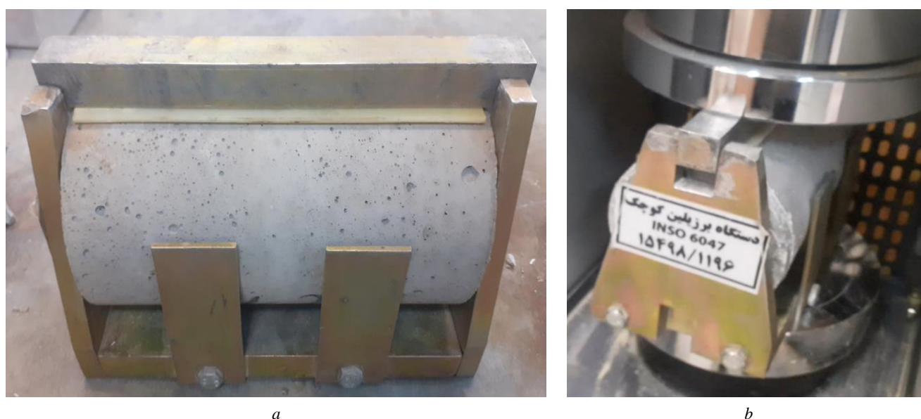
Figure 10. Tension test: a – tension test method; b – cylinder samples under compression machine
