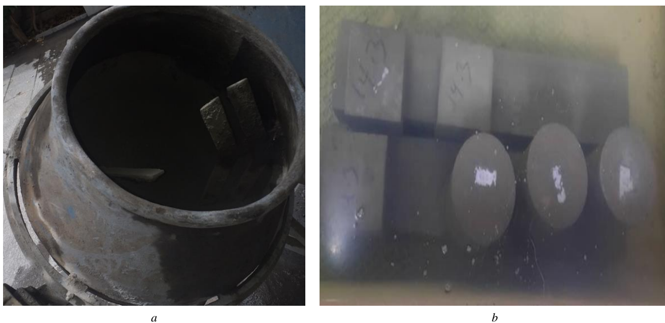
Figure 6. The pan mixture of laboratory (a) and molded concrete samples under water (b)
