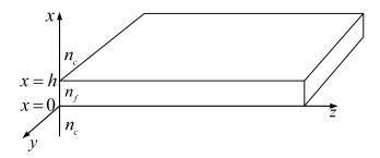
Figure 1. Symmetric three-layer dielectric waveguide
