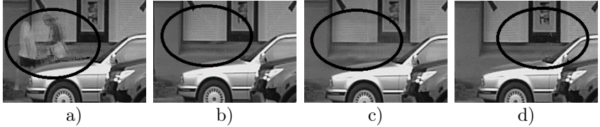
Figure 1. Typical visual artefacts in background models: a) running gaussian averaging, b) median, c) average, d) mixture of gaussians
