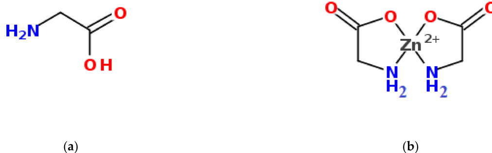
Figure 1. Chemical structures of glycine (a) and its zinc chelate compound—zinc glycinate (b).
