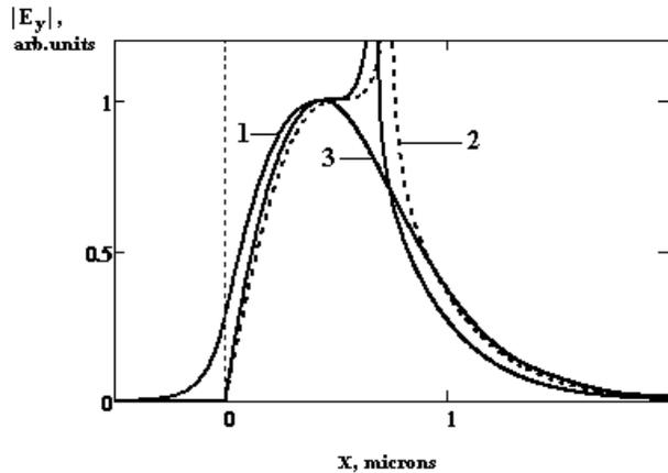
**Figure 3. Electric field amplitude of the TE-mode in a single-mode waveguide with Gaussian refractive index profile (3) calculated by various methods**
