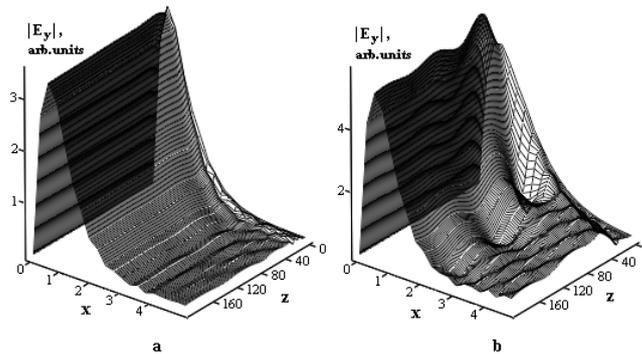
**Figure 1. Field pattern in the substrate of a single-mode waveguide with exponential refractive index profile (2) computed by the BPM. The input beam width  $w = 0.47 \mu\text{m}$  (a),  $0.65 \mu\text{m}$  (b). Distances along  $x$ - and  $z$ -axes are given in micrometers**
