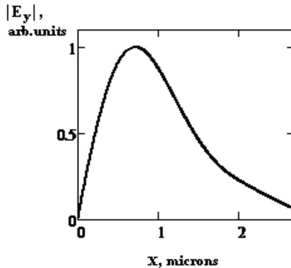
**Figure 4.** Electric field amplitude of the fundamental TE-mode in a multimode graded-index waveguide computed by the BPM for the refractive index profile evaluated on experimental data
