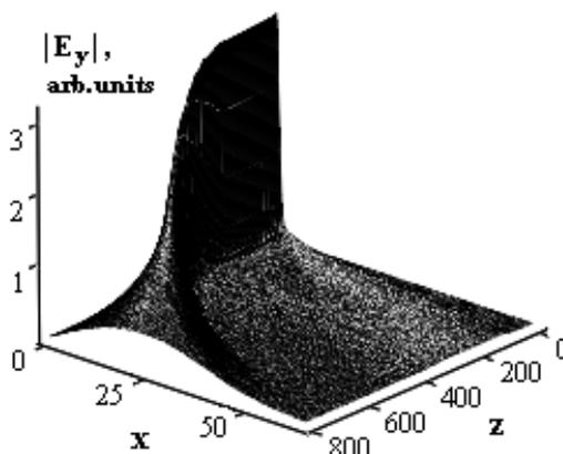
Figure 5. Field pattern of light radiation into the substrate of a graded-index single-mode waveguide with a tapered edge
