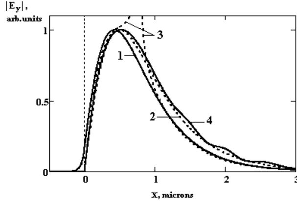
**Figure 2. Electric field amplitude of the TE-mode in a single-mode waveguide with refractive index profile (2) calculated by various methods**
