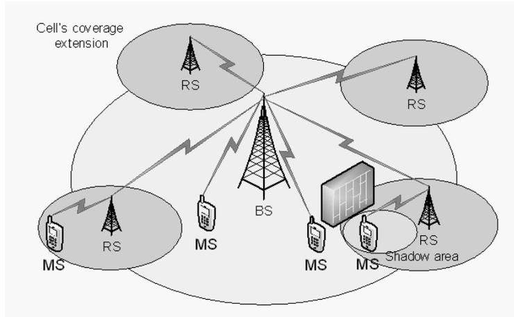
**Figure 1. The fixed infrastructure of relay-enhanced LTE-Advanced cellular networks**
