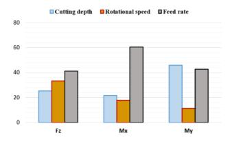
Figure 7. The Results of Taguchi approach for studying the effect of milling process parameters on the cutting forces and moments
