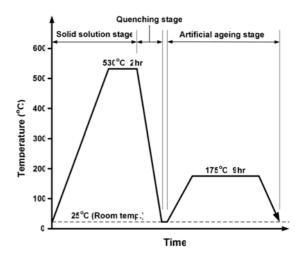
Figure 1. The conventional T6 heat treatment of Al 6061 alloy [18]
