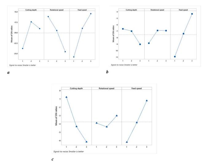
Figure 6. Means of SN ratios of different outputs under the impact of milling process parameters, including: a — mean of cutting force in the z-direction, b — mean of cutting moment around the x-axis; c — mean of cutting moment around the y-axis
