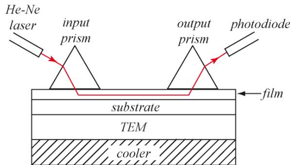
Figure 1. Optical scheme of the measuring system
