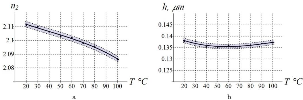
Figure 2. The dependence of the refractive index (a) and film thickness (b) on the temperature
