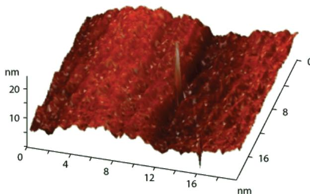
Figure 5. Micrograph of the surface of  $\text{TiO}_2$  films of a 3D image
