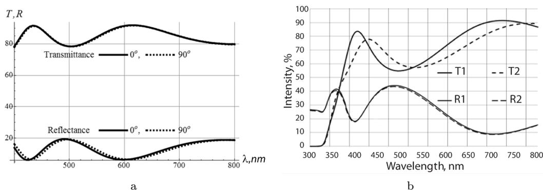
**Figure 3.** The transmission and reflection spectra of films: (a) — film thickness  $0.08 \mu\text{m}$ ; (b) — film thickness  $0.21 \mu\text{m}$
