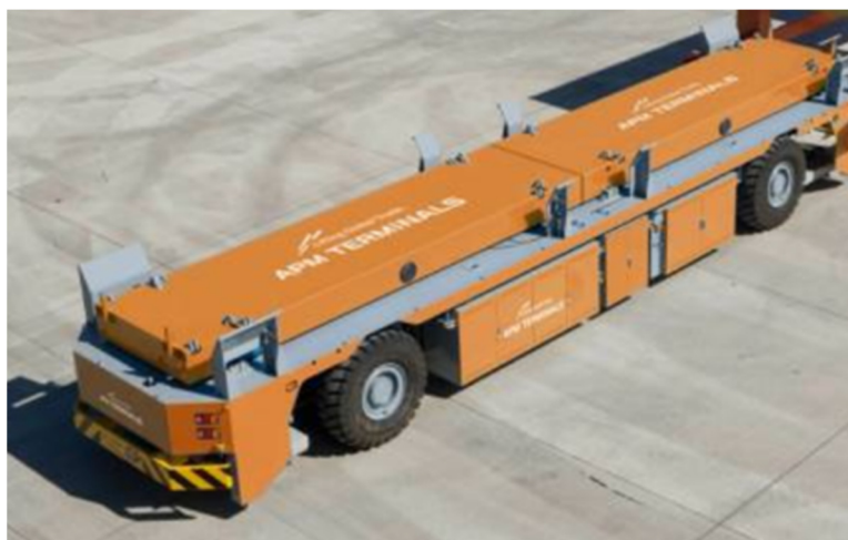
Figure 4. Unmanned, automatically guided vehicle.
