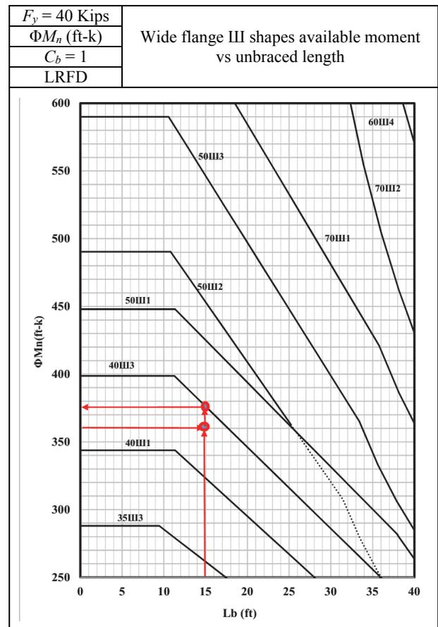
Figure 5.  $\Phi M_n$  vs  $L_b$  for optimal section
