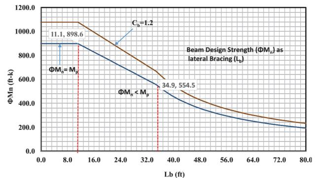
Figure 2.  $\Phi M_n$  vs  $L_b$  for 60III2
