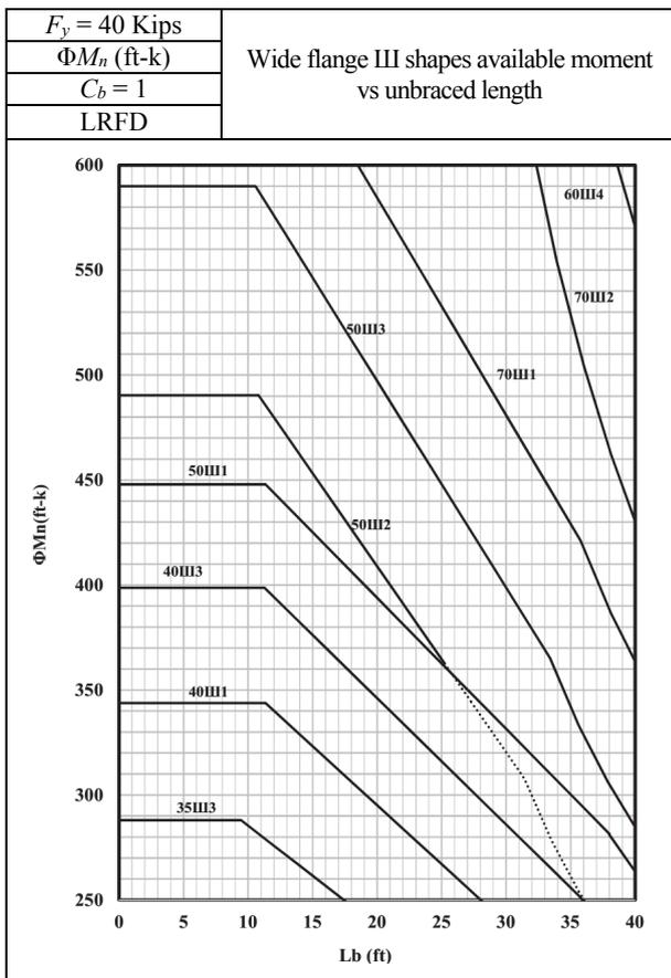
Figure 4.  $\Phi M_n$  vs  $L_b$  design chart
