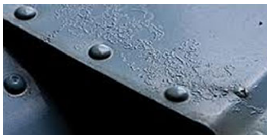
Fig. 4. Thread corrosion of painted aluminum [9]
