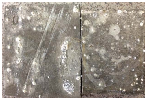
Fig. 1. Damaged surface of aluminum 6061 by corrosive environment [1]
