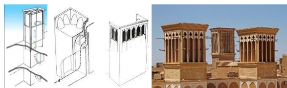
Pic. 5. Performance of wind deflectors
